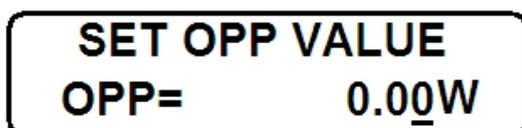
setting method is similar, and with the OPP (overpower protection) as a case, the function of the setting of the OPP is described. After entering OPP setting, the screen display the OPP.
