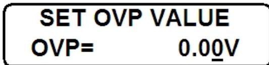
Press the ◀▶ key can adjust the position of cursor ,then rotate the adjusting knob to regulate the voltage to 30.00V.
