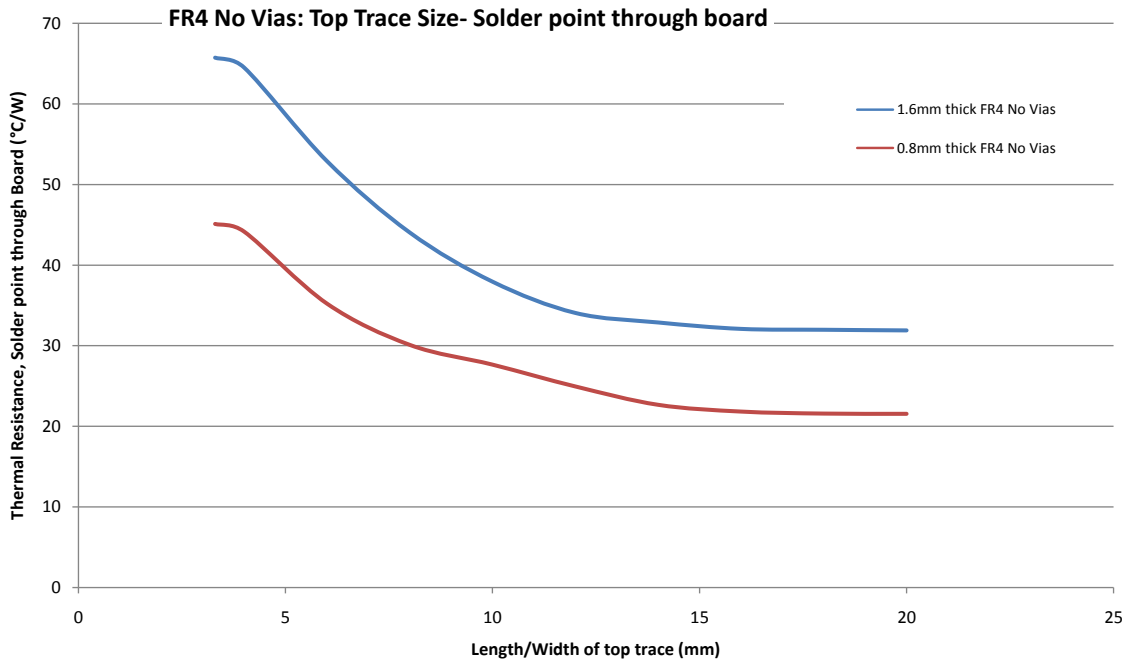
Chart 1: Thermal resistance for FR-4 PCB with no vias with varying thermal pad size
