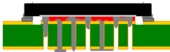
Figure 7: Solder voiding (not to scale)
